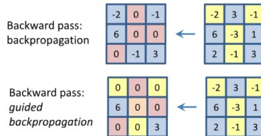
Figure 3.7: Backpropagation pass vs guided backpropagation pass. Extracted from Striving for Simplicity: The All Convolutional Net [20]
